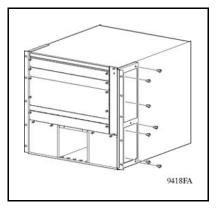
Measure the appropriate number of rack units of free vertical space inside the rack and mark the spot.
